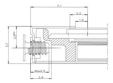
\*Mounting screw depth : Max 2.3mm \*Screw(4ea) Torque : Max 2kgf • cm
