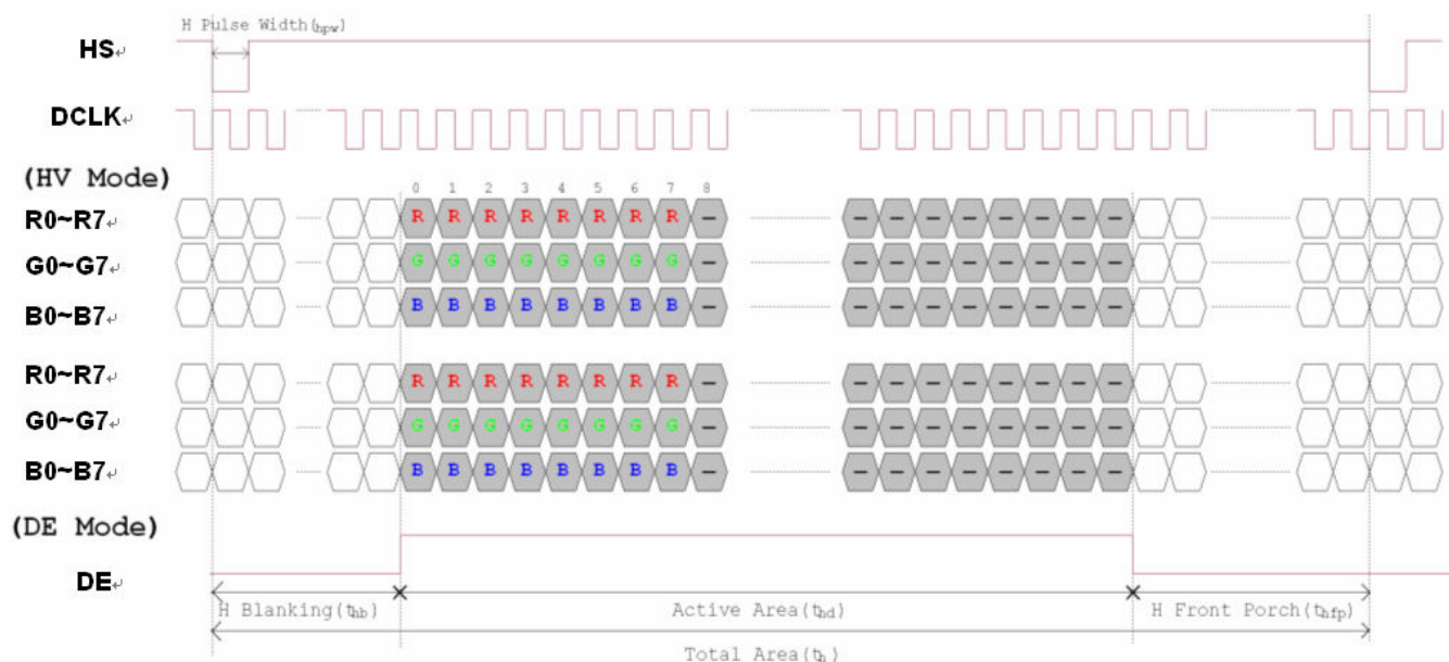
Figure 3. 1 Horizontal input timing diagram.
